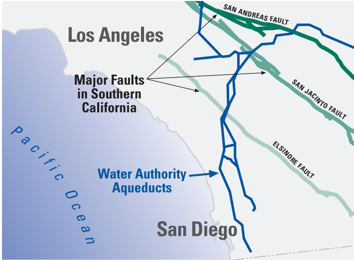
Water aqueducts serving San Diego County cross three major earthquake fault lines in Southern California.
